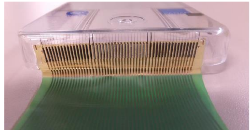
Corrected FPC and Electromagnetic Induction Junction
